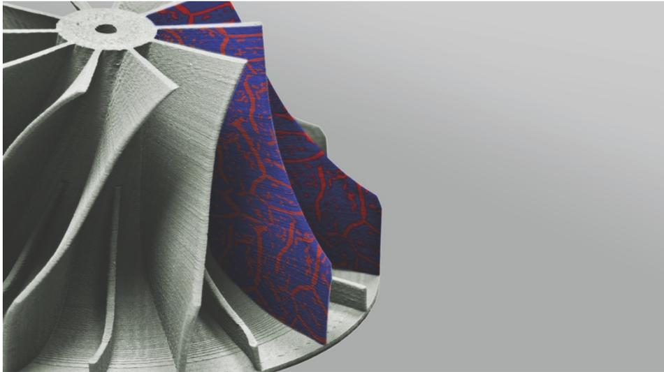
For the first time, scientists at Fraunhofer IWS printed 3D high-entropy demonstrator structures made of the Cantor alloy "CrMnFeCoNi" using the Fused Filament Fabrication (FFF) process. On the surface, the illustration shows an example of a particularly high-strength microstructure consisting of two phases as a planned further alloy system development.
